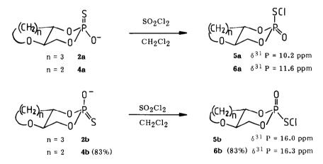
The configurational assignments of 5a, 5b, 6a and 6b were made by comparison of their  $^{31}P$  chemical shifts (positive downfield from 85% H<sub>3</sub>PO<sub>4</sub>) to those at 13.0 ppm (for P=O axial) and 9.2 ppm (for P=O equatorial) reported for the corresponding sulphenyl chlorides in the 4-methyl-1,3,2-dioxaphosphorinane series.<sup>10</sup>
